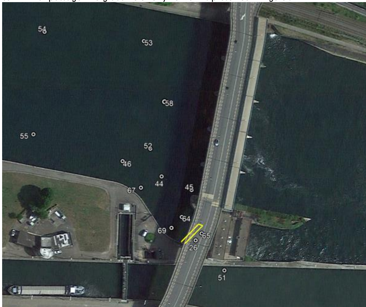
Figure 7 : 2D telemetry network installed at CHG (up) and CHR (down). Hydrophones 64, 65, 69 and 26 are covering the forebay.
