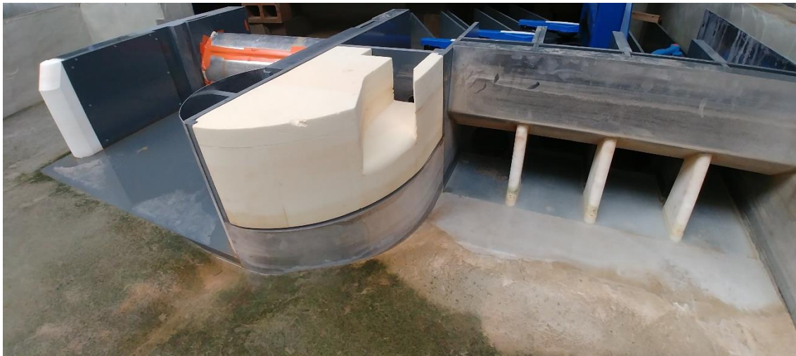
Figure VIII-11: Separation wall on Grands Malades model made using high-density foam (yellow material)
