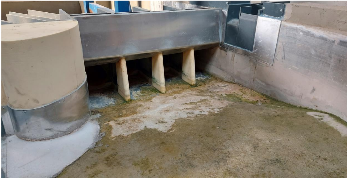
Figure X-8: Modified Grands Malades physical model to represent Lixhe HPP – View of intake channel from upstream.
