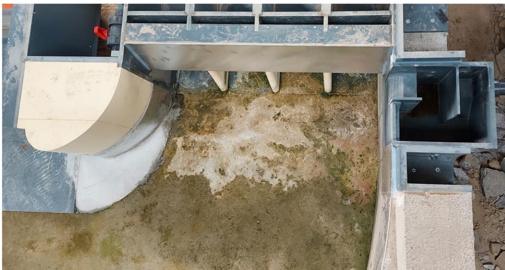
Figure X-9: Modified Grands Malades physical model to represent Lixhe HPP – Topview with the bypass on the right
