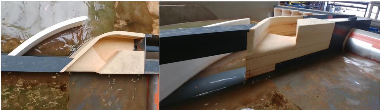
Figure IX-10: Initial geometry of fish passage intake at Ivoz Ramet
