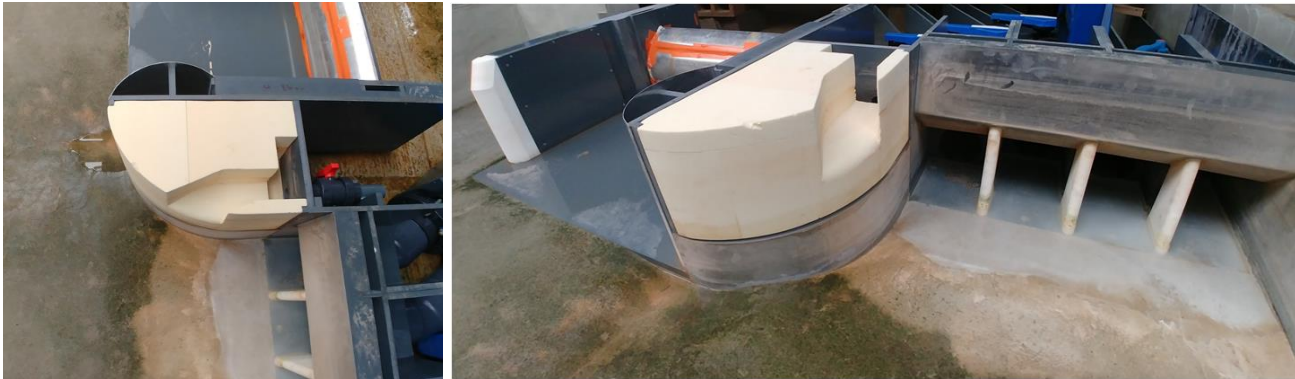
Figure IX-2: Initial geometry of fish passage intake at Grands Malades
