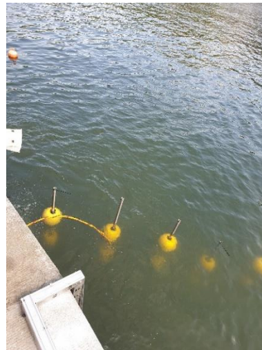
Figure 24 : Electrodes after cut with the marking of the water level before cut (colson)
