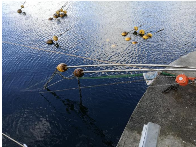
Figure 38 : Electrodes are out of water
