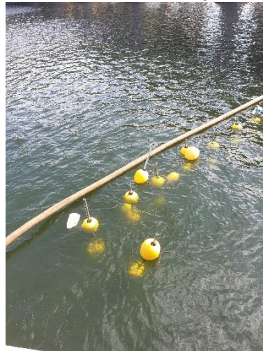
Figure 20 : The separation of the barrier from the water hose
