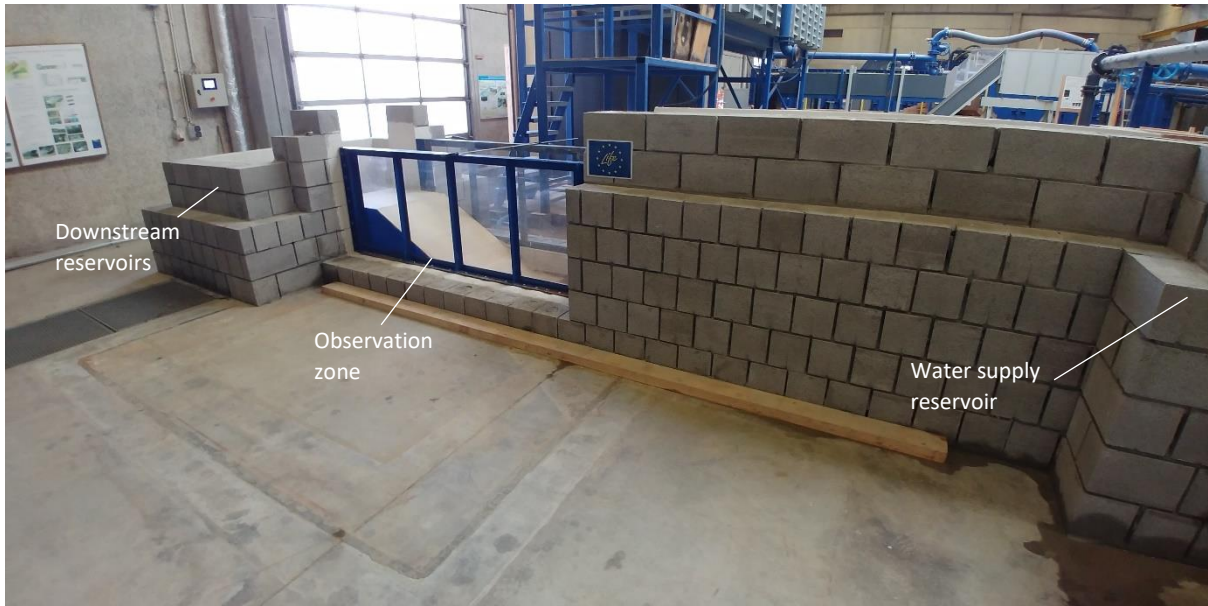
Figure 2 : Side view of the test flume with the left Plexiglas observation sidewall
