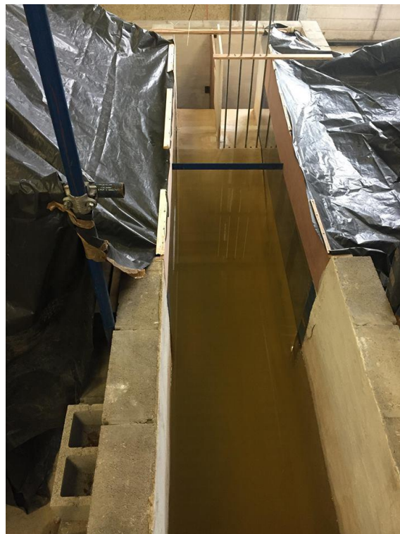
Figure 5 : Upstream view of the flume with a 10cm spacing rack on the crest of the right outlet
