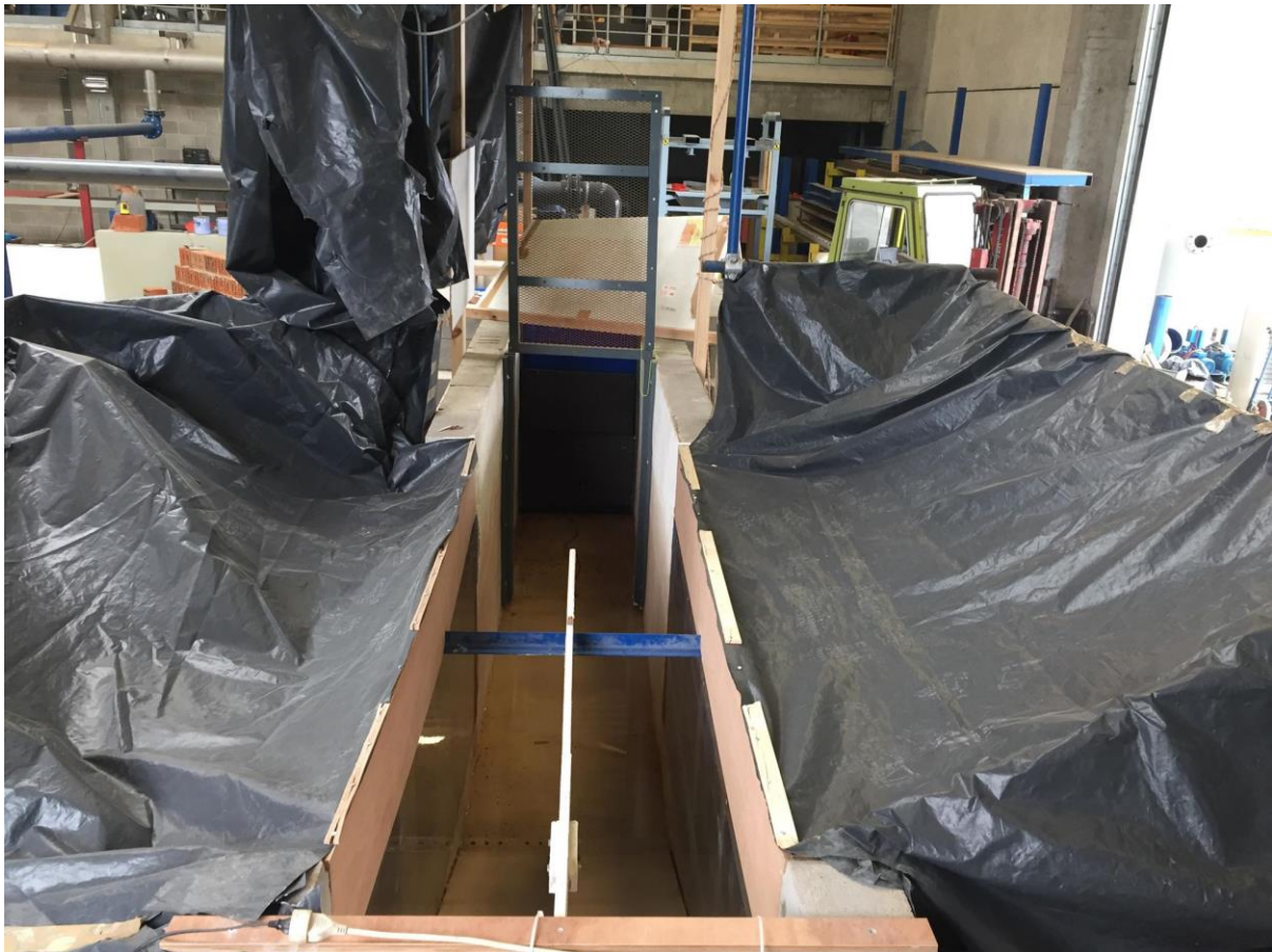
Figure 4 : Downstream view of the flume with plastic sheeting to hide observation sidewalls
