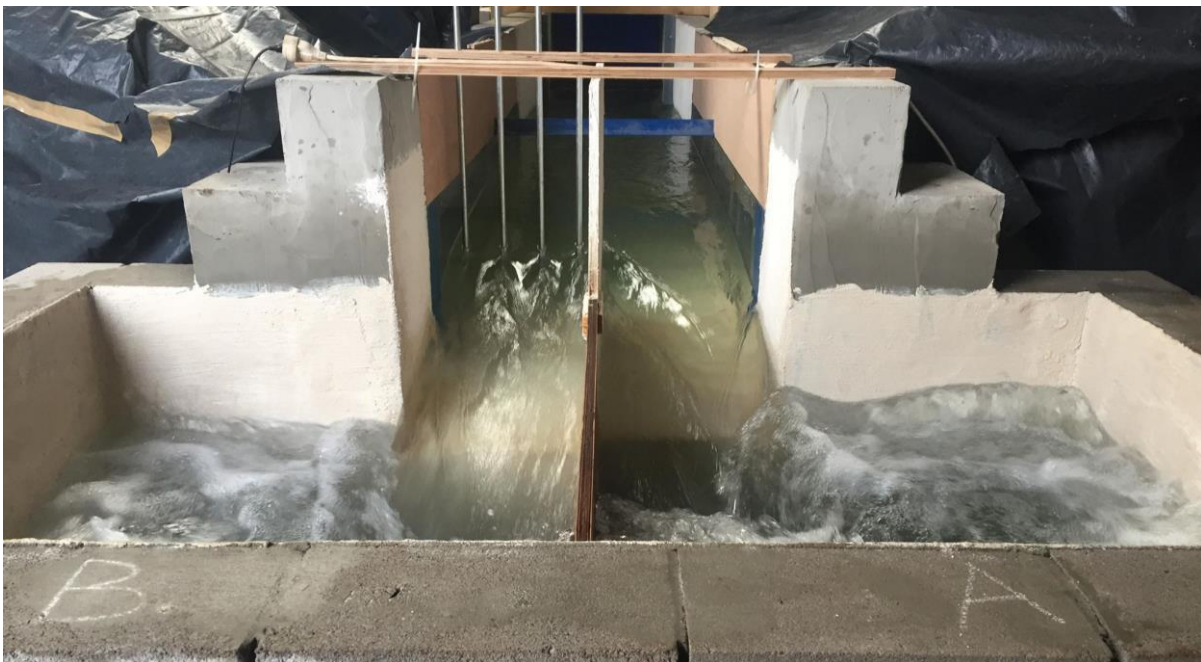
Figure 7 : Upstream view of the flume during a test with a rack bars spacing of 10cm in right outlet – Downstream reservoirs at the front
