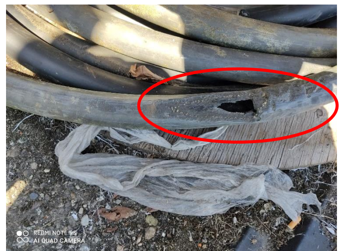
Damage to the bubble pipe at the bottom of the river
