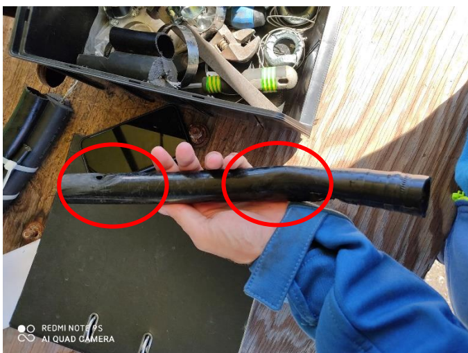
Breach and deformation of the air supply pipe
